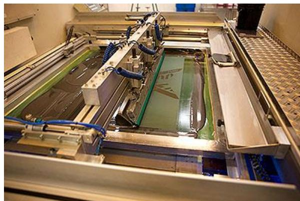
Direct digital printing can place the image directly onto the molded component at 180 impressions per minute. With screen printing, the IML needs to be placed into the molding tool cavity with an end-of-arm process with mold cavitation of 24 parts per every 30 seconds.
